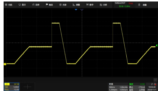
Sequence test output waveforms
